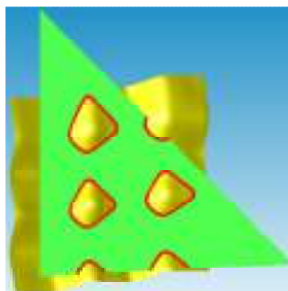
Fig. 7: Intersection between a triangle and an MLS surface resulting in multiple open branches and internal loops.
