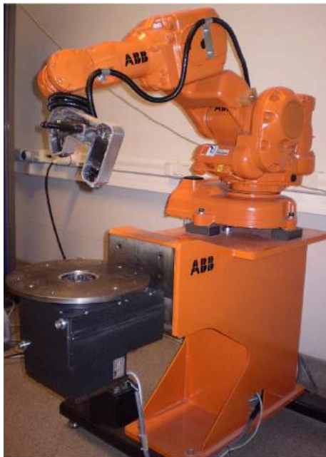
Fig. 1: Robot arm, turntable and laser profile scanner.
