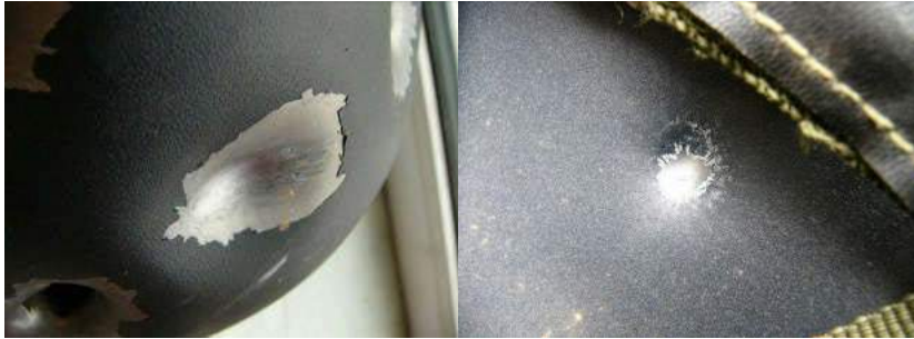
Fig. 1: Deformations on the exterior and interior surface of a steel helmet.
