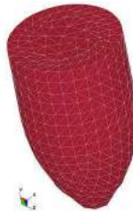
Fig. 6: The FE model of bullet.
