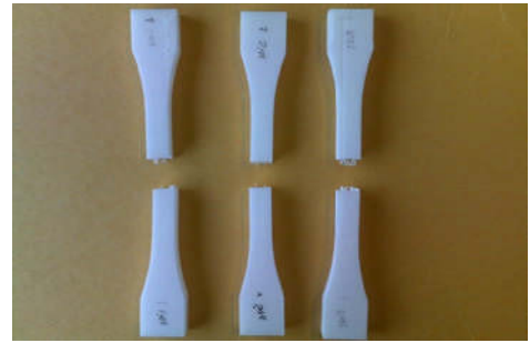
Fig. 2: The angle between the load direction (the center line) and the layer surface \theta . The right one shows the specimens failure in tensile tests.
