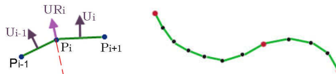
Fig. 4: (a) Determination of normal vector for a point, (b) Inflection point detection.
