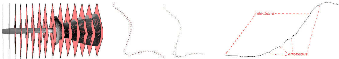
Fig. 14: (a) Screwdriver point cloud slicing, (b,c) Slice thinning, (d) Concavity change detection.
