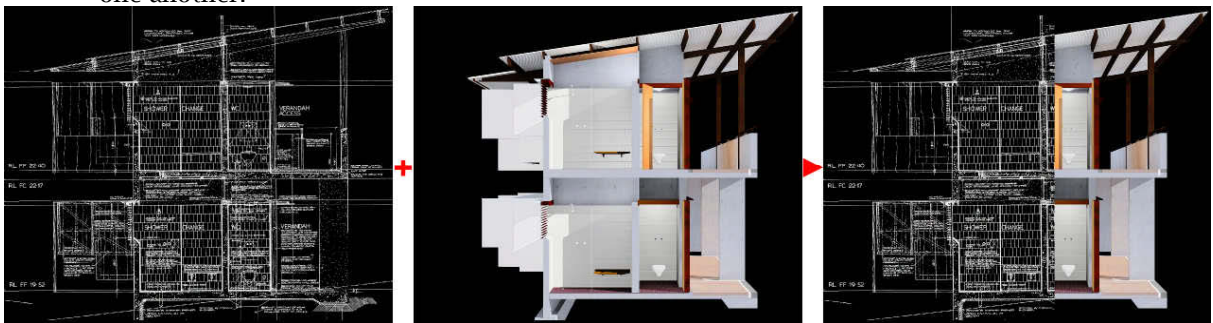
Fig. 2: Layering a construction drawing of Murcutt, Lewin and Lark's The Arthur and Yvonne Boyd Education Center and a digital model in interactive manner to increase Depth of Information - the whole could be more than the sum of its parts.
