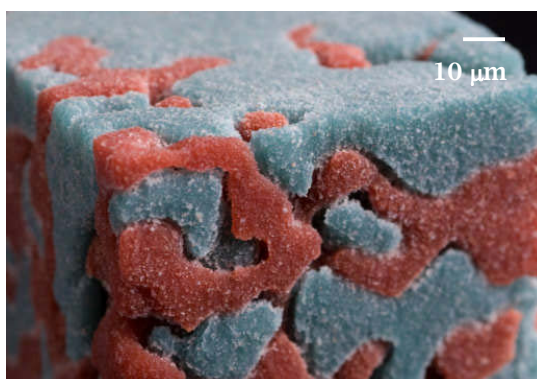
Fig. 6: Tissue scaffold prototype fabricated from CAD model in figure 5. Spaces in this scaffold design are for endothelial, epithelial, interstitial cell and their corresponding extracellular matrixes.
