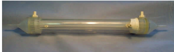
Fig. 5: 3D construct of the Initial FIF bioreactor after tests.
