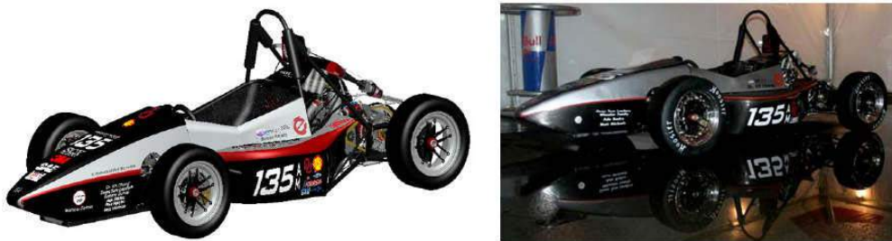
Fig. 10: Formula SAE race car designed and built by students: (a) Race car designed in Pro/ENGINEER , and (b) Race car revealed and on display.
