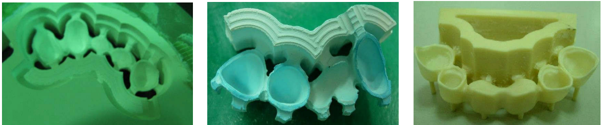
Fig. 3: The (a) Support bar, (b) Lingual type and (c) Ring-like type of support walls of tooth bridge.
