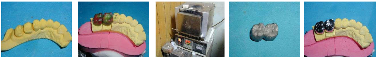
Fig. 1: Traditional process of tooth mold: (a) Impression, (b) Creation of wax base and sculpturing the shape, (c) The lost-wax casting process, (d) The Sand blasting process, (e) The polishing process.
