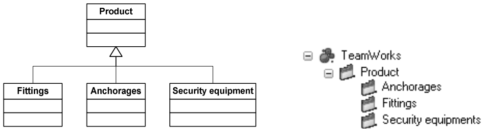
Fig. 10: UML class diagram and tree-view of the product family.
