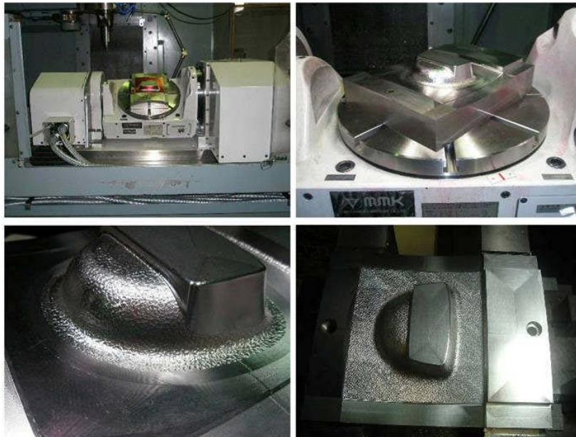
Fig. 9: The die under and after milling.
