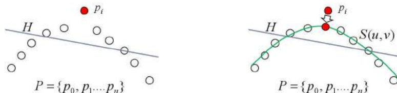
Fig. 13: Smoothing by fitting: (a) Referenced plane H , (b) Quadric surface S .
