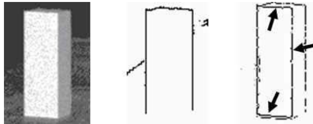
Fig. 6: Types of feature points: (a) Brightness image, (b) Silhouette lines, (c) Internal edges.
