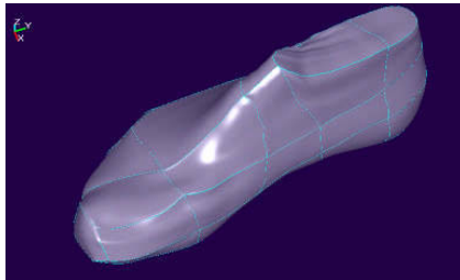
Fig. 7: (a) Modified shoe last, (b) comparison of original last, the foot and modified last.
