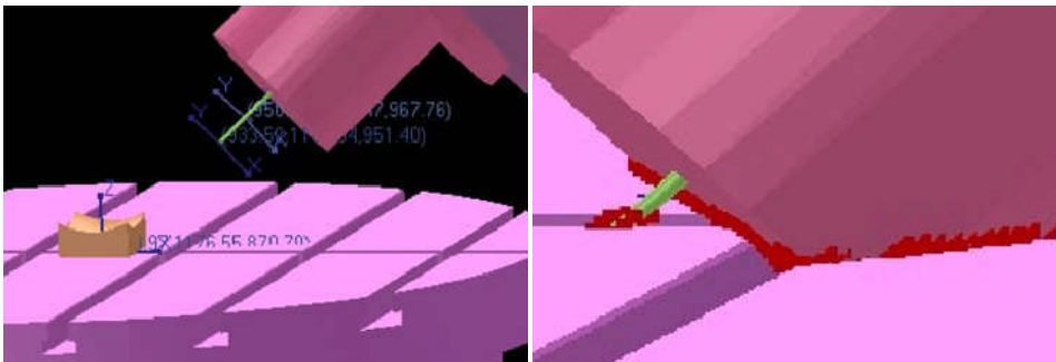
Fig. 5: Collision detection, for a five-axis virtual machine tool: (a) A snapshot of a virtual machine tool, before collision, (b) Collision occurs between the tool-spindle and the worktable. The collision area is marked with deeper color.
