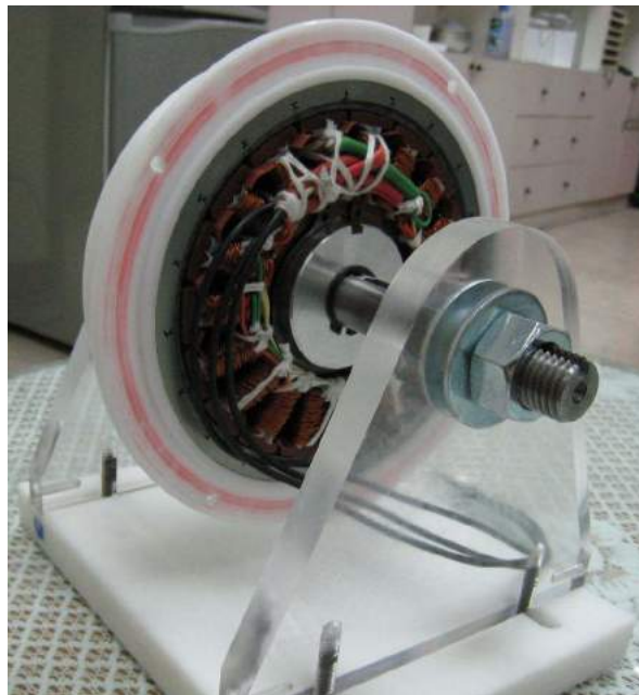
Fig. 14: The prototype of Case I for the proposed BLDC motor.
