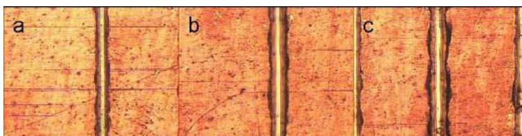
Fig. 19: The top view for different depth of cut (a) 5 \mu\text{m} depth of cut; (b) 10 \mu\text{m} depth of cut and (c) 15 \mu\text{m} depth of cut (100X).
