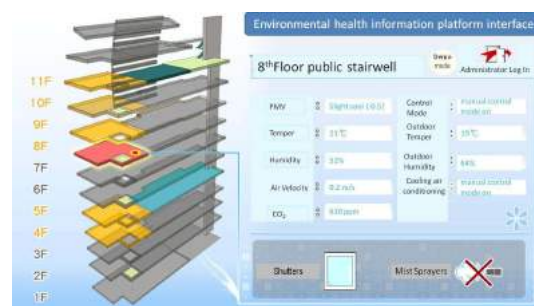
Fig. 10: Environmental information display interface in the Fu-An Memorial Building environmental health information platform.
