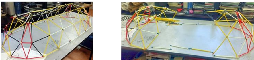
Figure 9. Physical model (obtained by 3D printer) of the rectangular-based structure.
