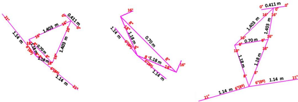
Figure 3: Final design of the prototype Lattice corner from geodesic dome transformation, frequency 2.
