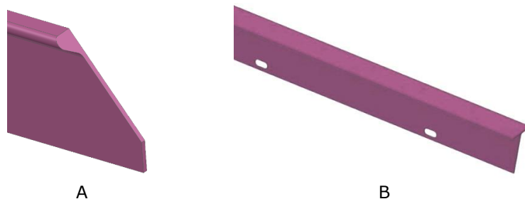
Figure 2: A left-end cut on a 3D model of a stiffener (A) and ventilation holes in the stiffener's middle section (B).
