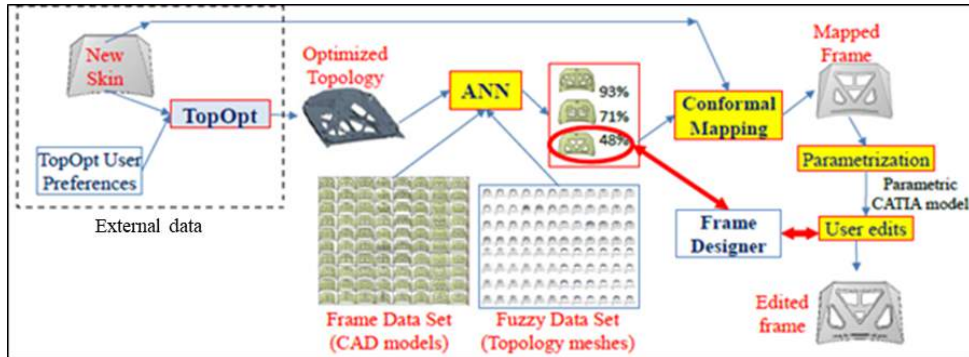
Figure 5: Workflow of Data-centric Hood Frame Design
