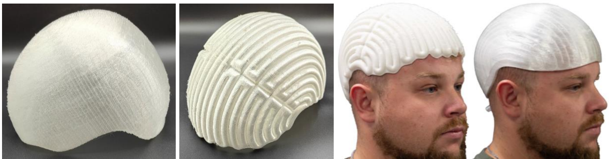
Figure 9: 3D printed generic outer shell (left), standard printed cooling cap (left, mid), Customized cap (right mid), bespoke CAD customized cap (right).
