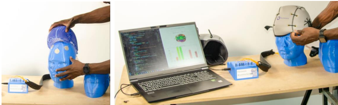
Figure 5: Testing wearable design combinations on Pressure Sensitive 3D Printed Head Rig.
