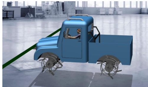
Figure 4: The paddy sprayer.
