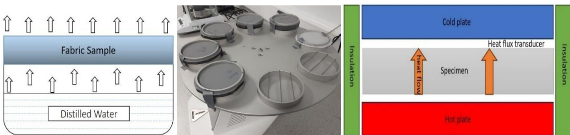
Figure 3: Thermal conductivity testing and water permeability testing machines.
