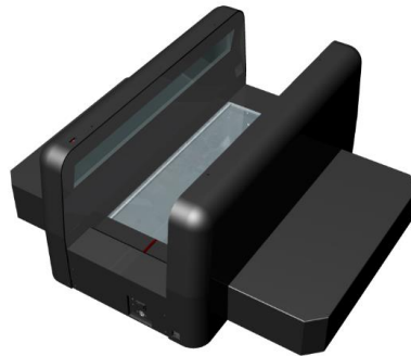
Figure 3: INFOOT 3D Foot Scanner for feet data acquisition.
