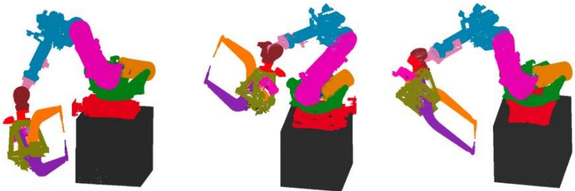
Figure 17: Segmentation of virtual point clouds into robot links.
