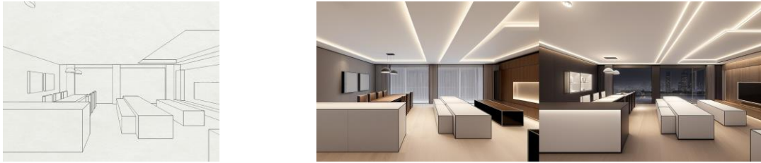
Figure 2: The AI-generated images from a low LOD model: (a) A low-LOD model applying the "Pen" display mode in Rhino for generating a canny controlling map, (b) two generated images by the canny ControlNet model.
