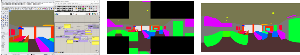
Figure 5: The generation of a panoramic segmentation map from a scene in Rhino: (a) Setting the custom display mode for ADE20K semantic segmentation, (b) the generated cubic projection images, and (c) the converted equirectangular projection image.
