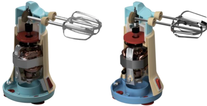
Figure 7: Cross-sections of virtual replicas of the hand mixer assembled from 3D scanned mesh components (left) and CAD-modeled feature-based components (right).
