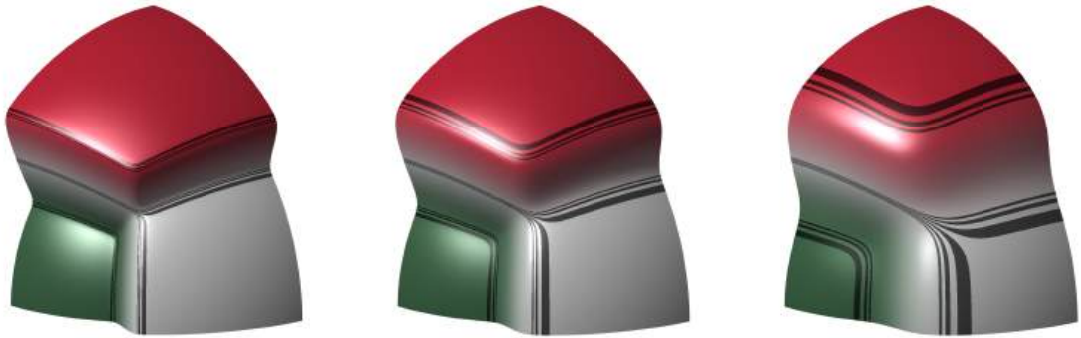
Figure 8: Visualizing the error of the spherical subsurfaces for varying smoothness. A stripe corresponds to about 0.01 difference in radial distance. (The red radius is 6, white is 5 and green is 4.) p = 32, 16, 8 .
