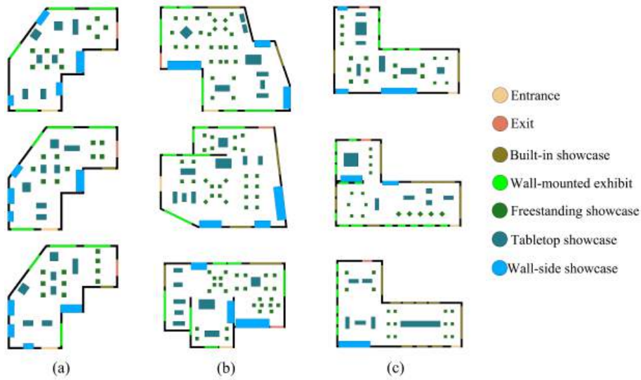
Figure 10: Various results from the proposed method. (a) Same input outline and requirement list. (b) Different input outline and same requirement list. (c) Same input outline and different requirement list.
