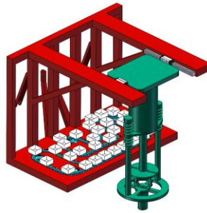
Figure 9: Conceptual Design-2 of the tractor-based automatic soil sampling device.
