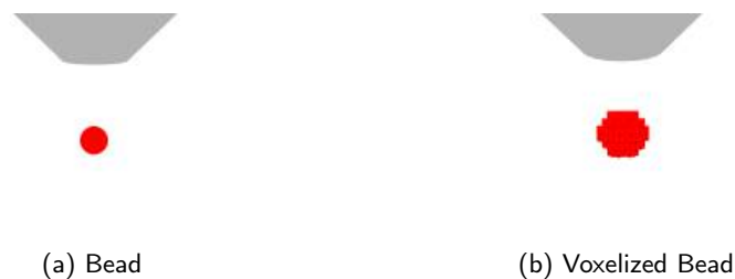
Figure 12: Comparison of Bead Geometry Before and After Voxelization Under the Deposition Head
