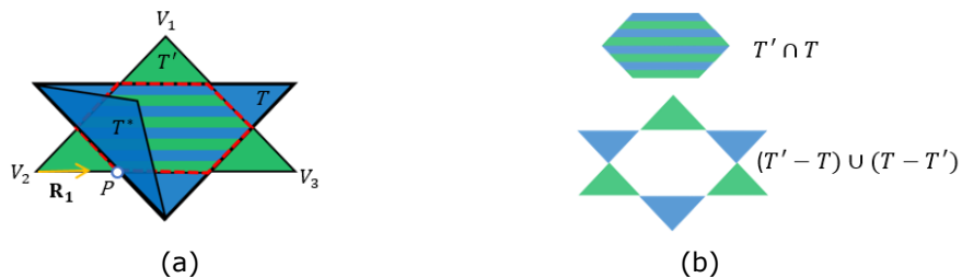
Figure 6: (a) The triangle T' is coplanar with T , and T^* is an adjoint triangle of T and is not coplanar with T' and T . At the boundary of the coplanar region, the ray R_1 emitted along the edge V_2V_3 intersects with T^* at point P . (b) The coplanar region T' \cap T and noncoplanar region (T' - T) \cup (T - T') .
