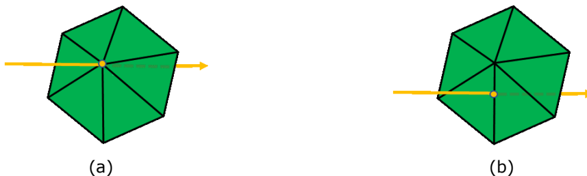
Figure 8: The rays intersect with multiple triangles at one point. (a) The intersection point is on one vertex. (b) The intersection point is on one edge.
