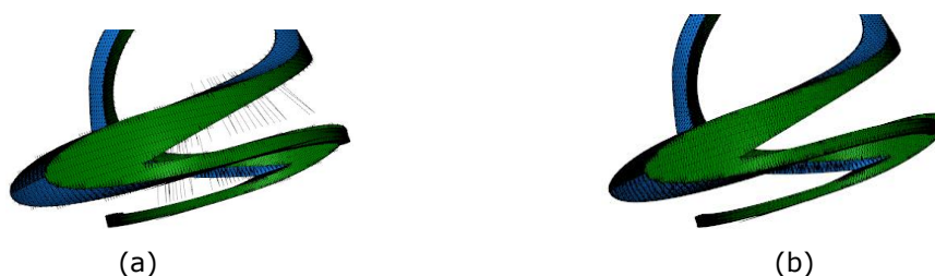
Figure 10: A real-world illustration. (a) Due to calculation errors, the result is a lot of tiny triangles. (b) After taking measures, the right result is obtained.
