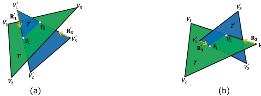
Figure 4: The two most common triangle-triangle intersection cases. The triangles T' and T belong to two input models. (a) The rays \mathbf{R}_1' and \mathbf{R}_3' emitted from T' intersect triangle T at points P_1 and P_2 , respectively. (b) The ray \mathbf{R}_1 emitted from triangle T' and the ray \mathbf{R}_3 emitted from triangle T intersect at points P_1 and P_2 , respectively.
