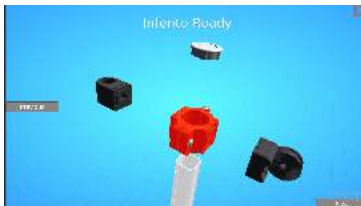
Figure 9: Exploded view, handlebar junction
