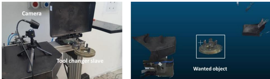
Figure 17: Left: acquisition test of the tool changer slave; Right: acquisition example carried out in NEURAL mode at almost 1 m distance along Z.
