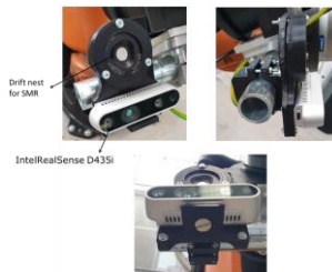
Figure 13: Complete system: robot, camera and SMR.
