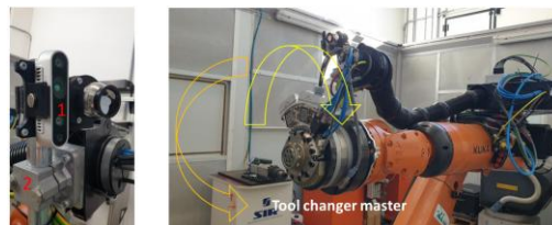
Figure 14: Assembly of the SMR for calibration and identification of the two planes for the axis calculation.
