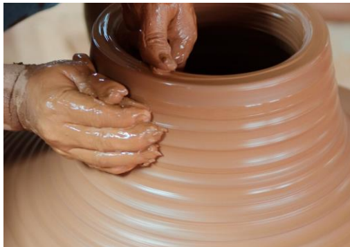
Figure 2: Li Pottery craftsmen pull blanks by hand.
