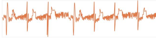
Figure 1: ECG waveform with power frequency interference signal.
