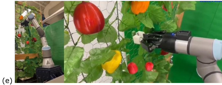
Figure 17: (a – e) Robot trajectory to harvest detected cucumbers based on received position data in a 3D printed artificial greenhouse
