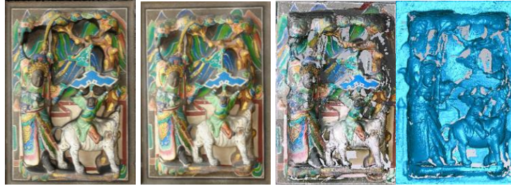
Figure 5: 3D model of a stone sculpture panel using Zephyr® (left) and Postshot® (middle), comparing to former 3D scanned result (right).
