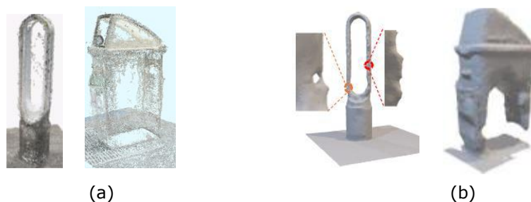
Fig. 1: Point clouds acquired by a mobile device and generated 3D meshes: (a) Low-quality point clouds and (b) Meshes generated by existing methods [23].
