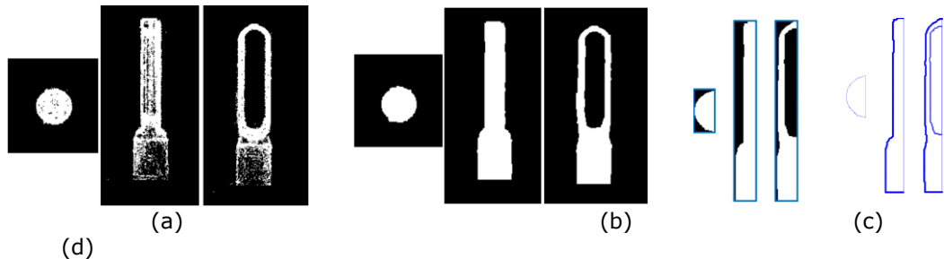
Fig. 4: Projected image and contour polyline: (a) Projected image, (b) Silhouette image, (c) Half image, and (d) Contour point sequences.
