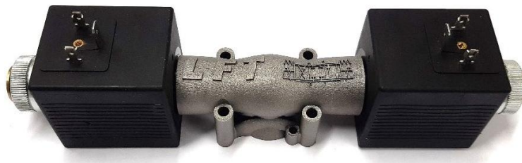
Figure 1: 3D printed hydraulic valve (size 3 according to CETOP), designed using TO and extensive CFD testing.
